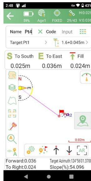
*For the Z1 receiver, you can use the IMU Stakeout feature. In IMU Stakeout, you can turn on the IMU feature without keeping the receiver perpendicular to the ground. The maximum tilt angle is 60°.*
