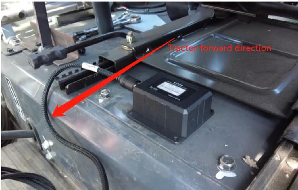
Figure 2.1.24 Gyroscope installation
