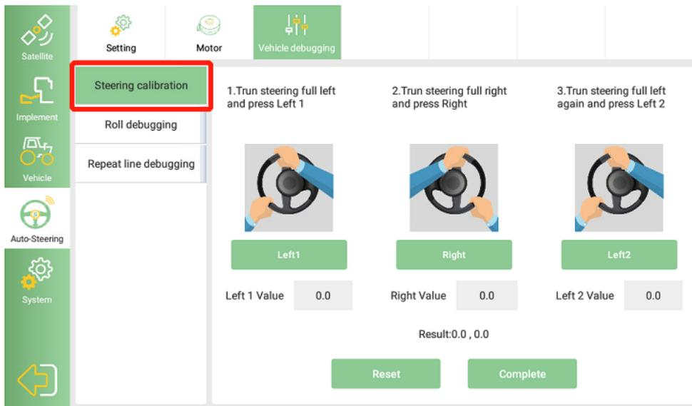
Fig 2.2.8 Vehicle calibration interface
