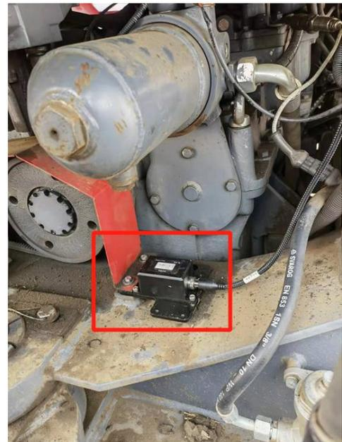
Figure 2.1.36 Gyroscope on articulated tractor
