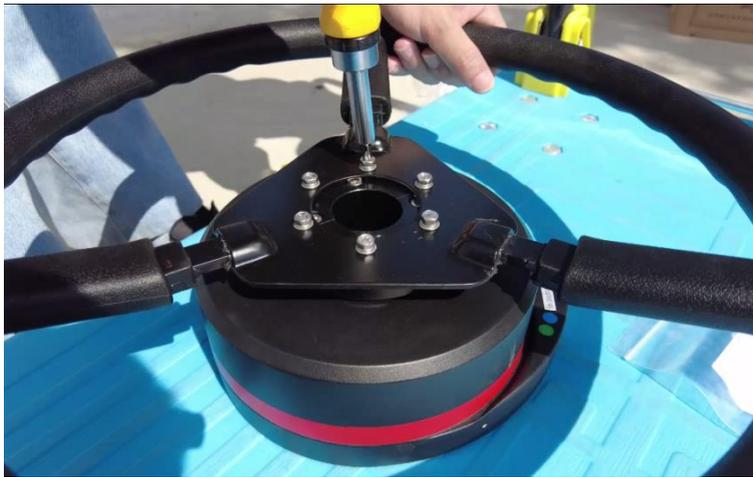
Figure 2.1.3 Steering wheel fixing
