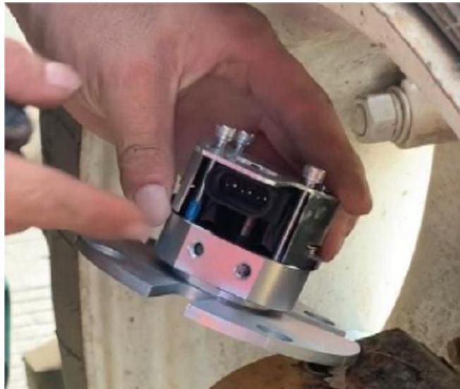
Figure 2.1.11 Mounting angle of the angle sensor
