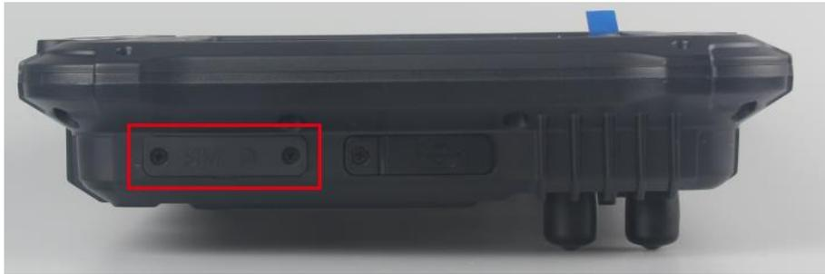
Fig 2.2.17 SIM card slot
