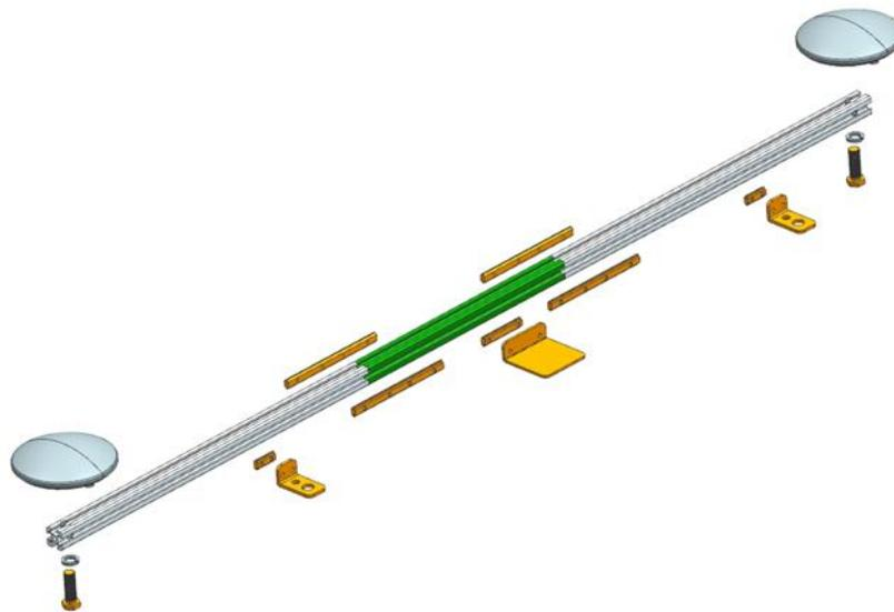
Figure 2.1.15 Assembly diagram of dual antennas
