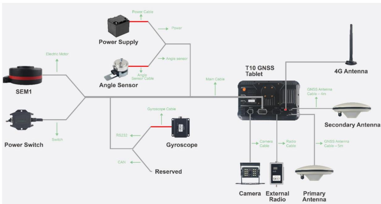
Figure 2.1.28 Cable Connection Diagram
