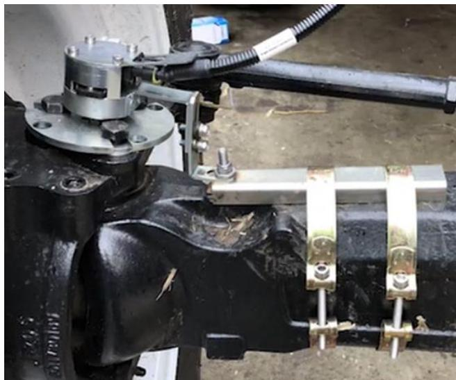
Figure 2.1.14 Installation example of angle sensor
