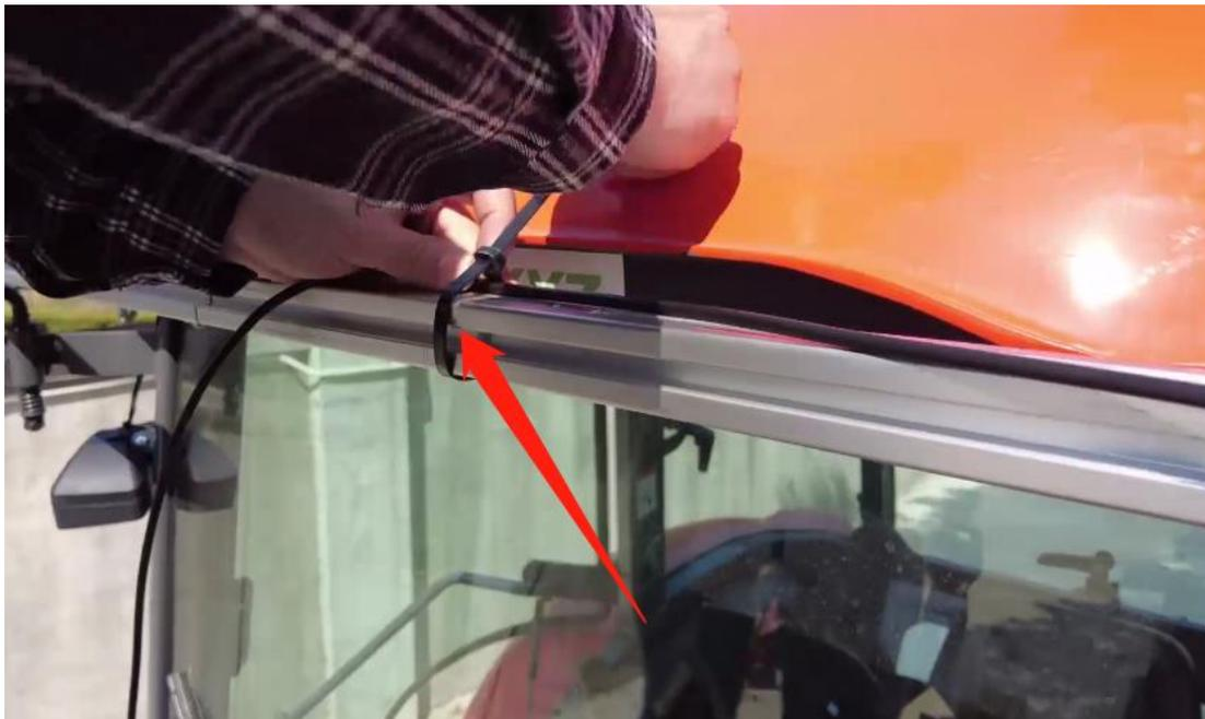
Figure 2.1.20 Antenna cables fixing
