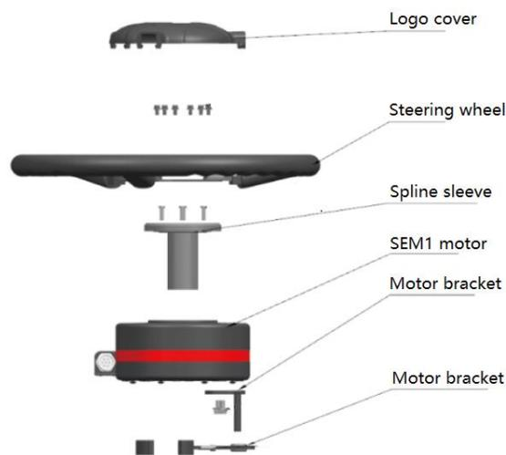
Figure 2.1.1 Assembly diagram of SEM1 motor wheel
