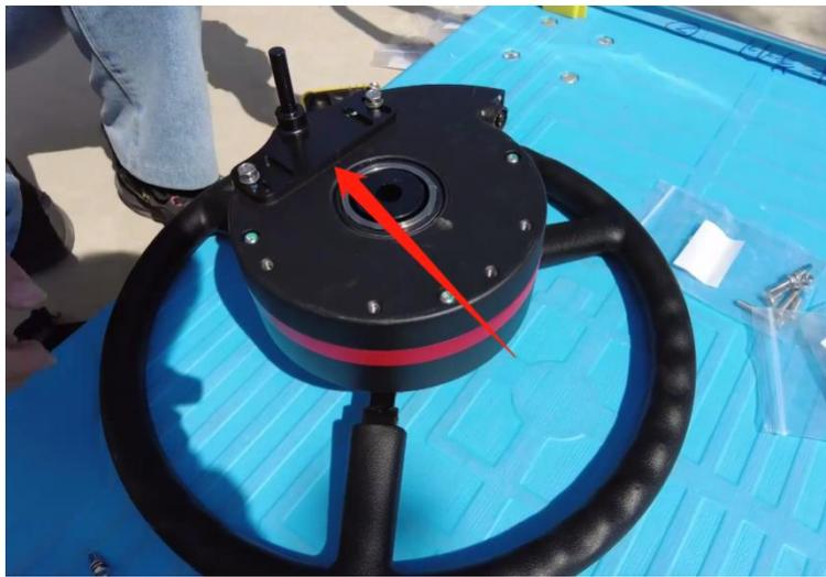
Figure 2.1.4 Motor bracket fixing
