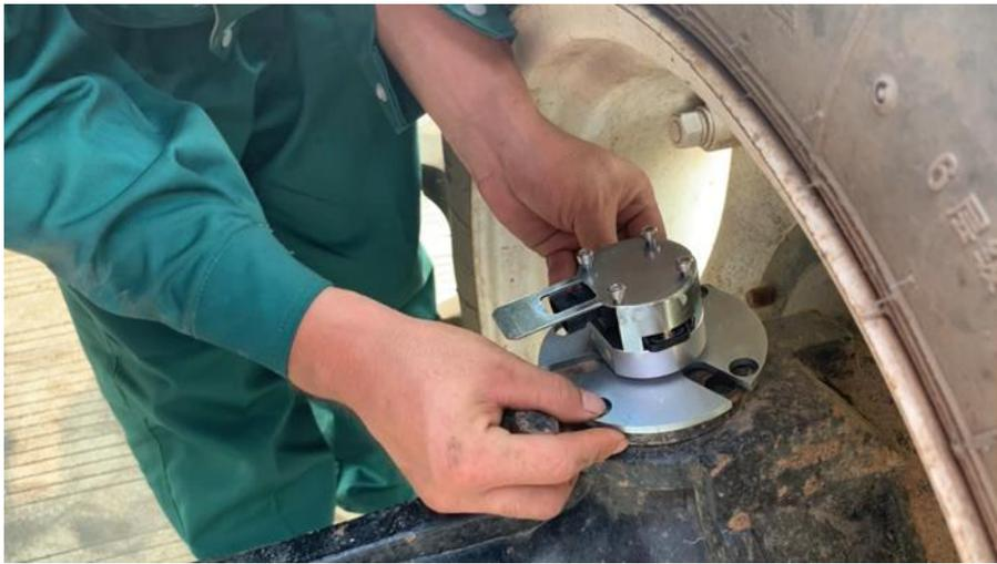
Figure 2.1.12 Install the parts to fix angle sensor
