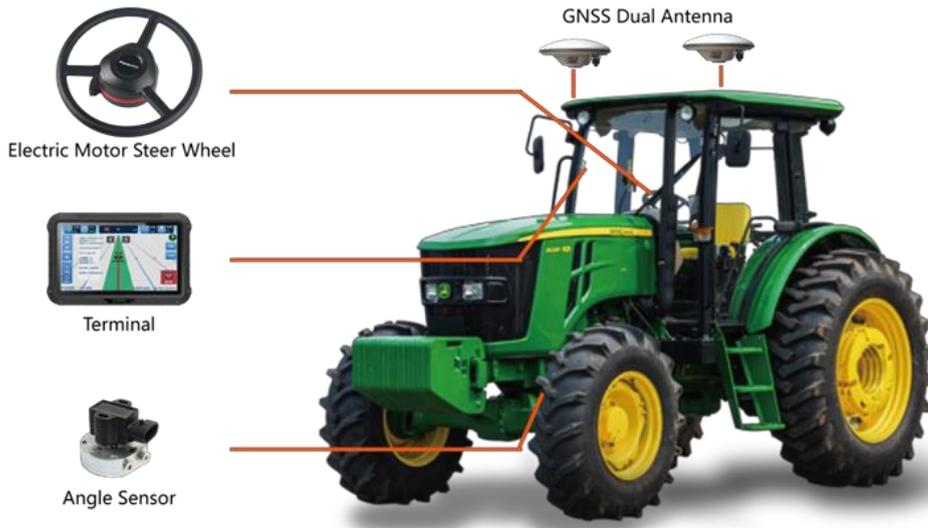
Figure 1.2 Sagro100 Automated Steering System structure
