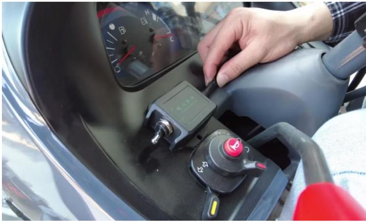
Figure 2.1.26 Power switch installation
