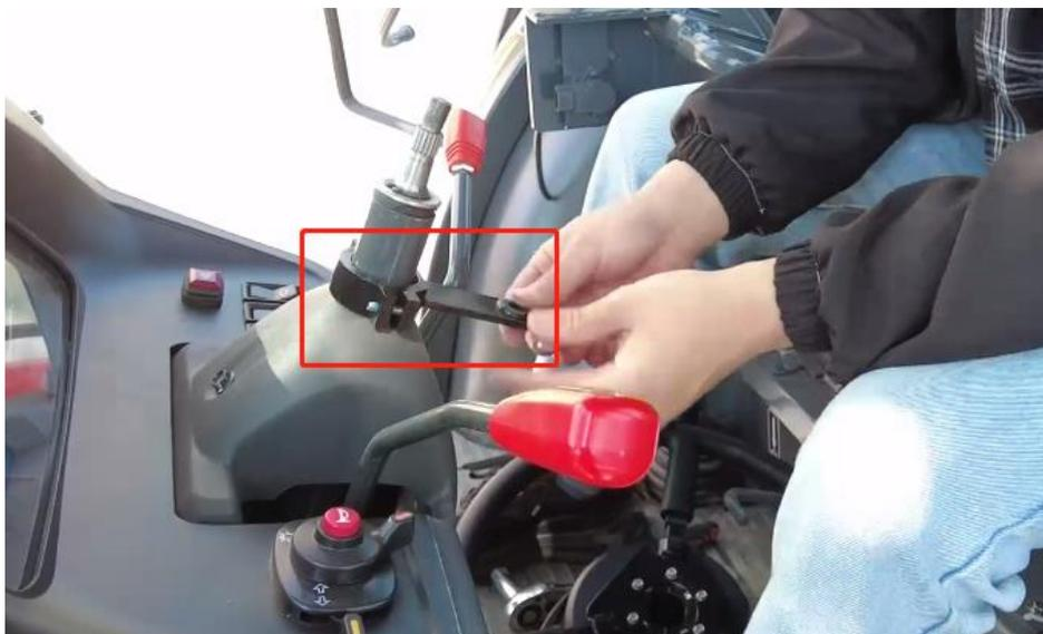
Figure 2.1.5 Motor bracket fixing
