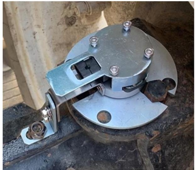
Figure 2.1.13 Fix angle sensor
