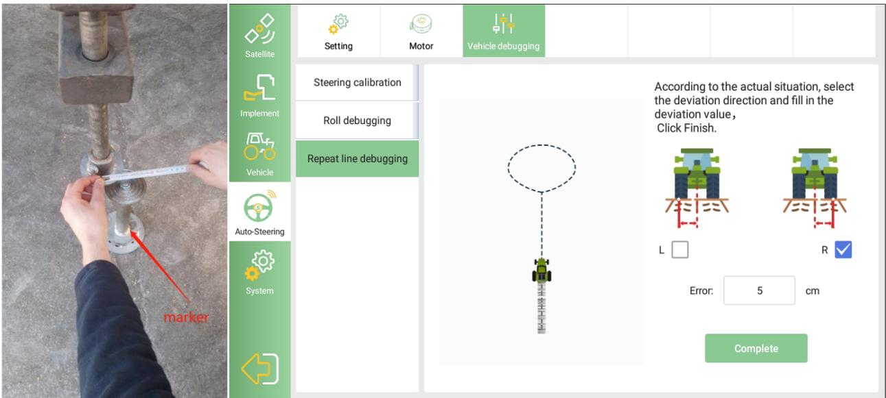
Finally, test the performance of it. If you find when your speed get higher, the offset change to bigger sometimes. You can system>> auto steering>>motor and adjust rotating speed. When you choose a higher speed, it should be reduced appropriately.
