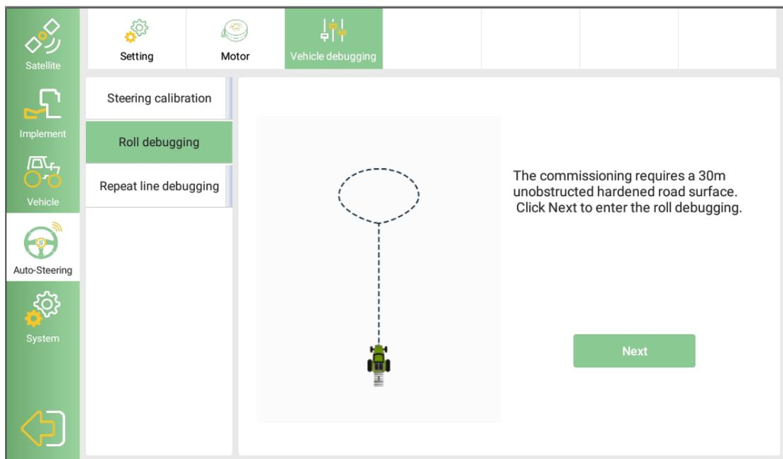
**Note: when you step 2 and step 3 for roll debugging, please stop in the red frame and wait collection finish, then drive.**
