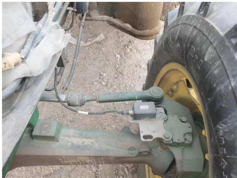
Front Wheel IMU Installation
