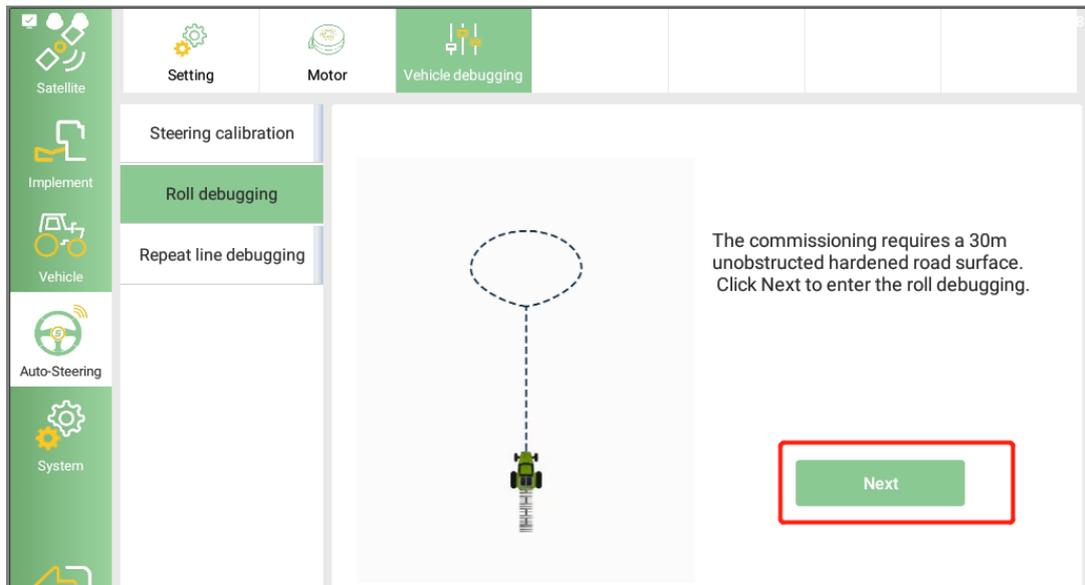
**Note: when you step 2 and step 3 for roll debugging, please stop in the red frame and wait collection finish, then drive.**
