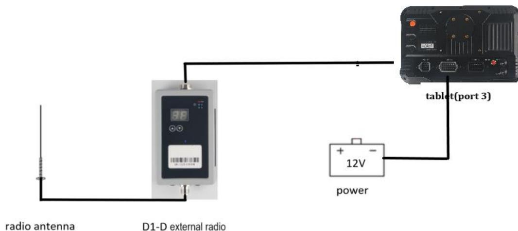
Then go to System >> Satellite >> Connect >> External Data interface, wait a few seconds it will run the extra module successfully, you should click the channel to configure the frequency and protocol, and click
