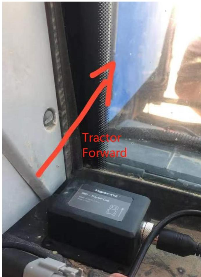
Tractor Cab IMU installation
