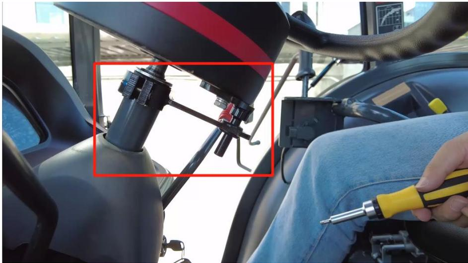
Motor exterior fixing
