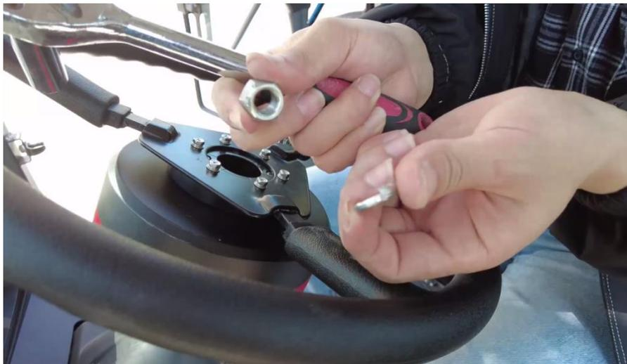
Motor shaft fixing -1
