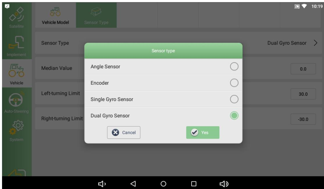
Return to the main interface and perform a self-check in the Status, the Dual Gyro Sensor should be normal.
