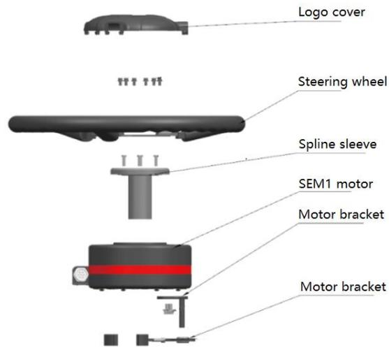
Assembly diagram of SEM1/SEM2 motor wheel
