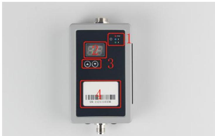
Indicators: three indicators, red - power indicator, blue - data upload indicator, green - data download indicator (when working normally, the indicator blinks red, green and blue in sequence)
