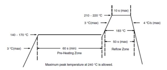
**Note**: For secondary assembly reflow soldering, we recommend that the module be placed in the final reflow process in the double-sided design application, and the module shielding cover should be placed upwards. We recommend the user a one-time reflow process. Please refer to
